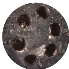
Injector before P.i. treatment.
