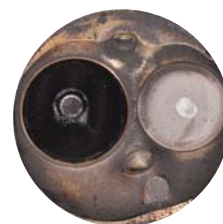
Cylinder head after one P.i. treatment.
