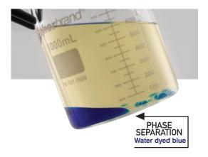
Phase separation is when ethanol/water mixtures fall to the bottom of fuel tanks and containers. leading to lean-burn conditions.
