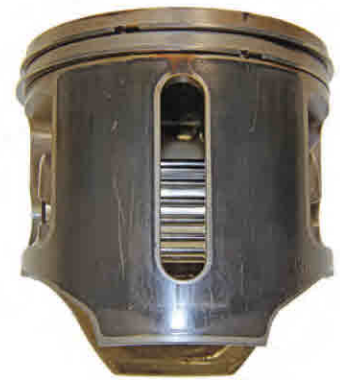
The Arctic Cat C-TEC engine injects oil into the crankcase through a slot in the piston. This setup, according to Arctic Cat, improves performance, emissions and fuel economy.
